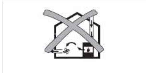
Fig. 4.1 Exhaust air installation – not permitted
